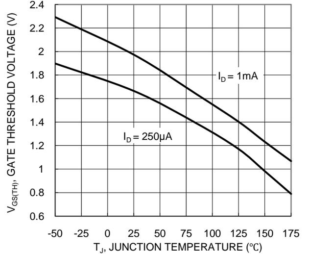
Figure 8. Gate Threshold Variation vs. Junction Temperature
