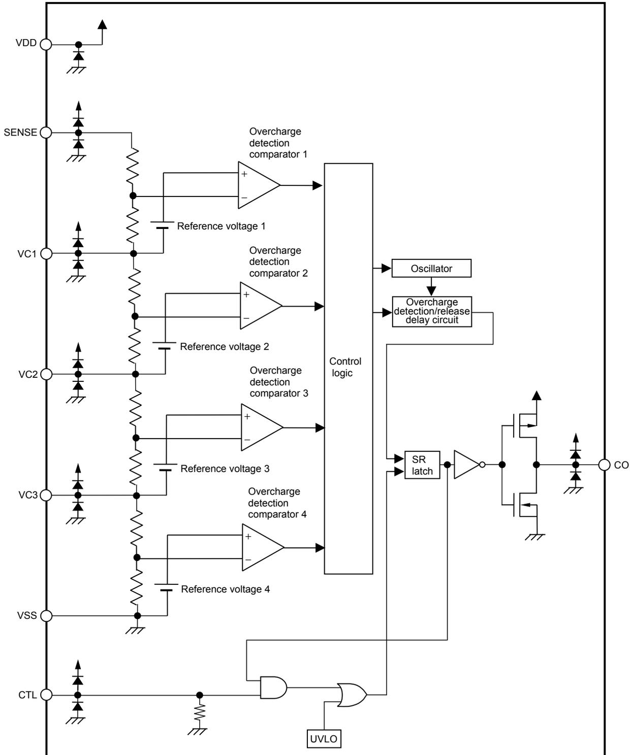
**Remark** The diodes in the figure are parasitic diodes.
