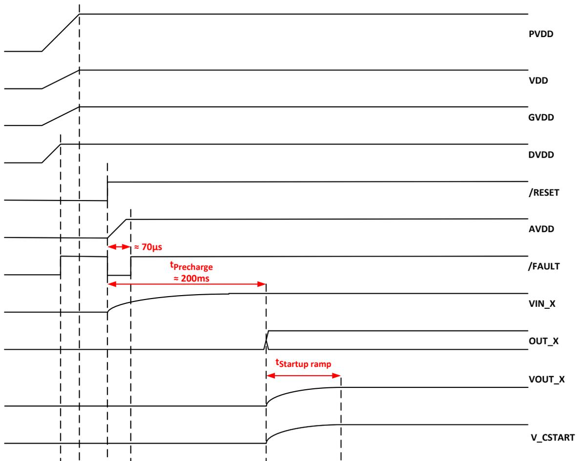
**Figure 30. Startup Timing**
