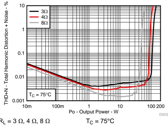
Figure 3. Total Harmonic Distortion + Noise vs Output Power
