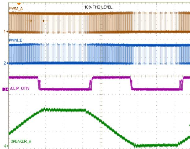
Figure 25. Signal Clipping PWM and Speaker Output Signals
