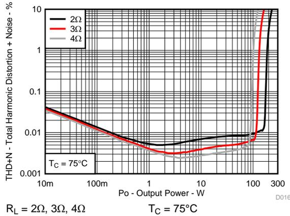
Figure 16. Total Harmonic Distortion+Noise vs Output Power
