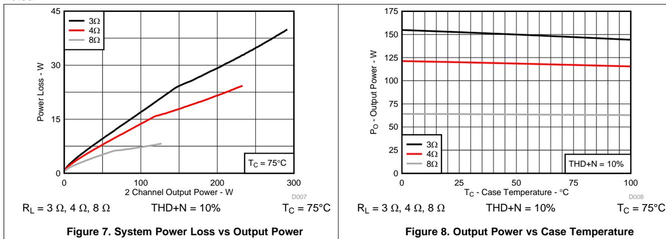
Figure 7. System Power Loss vs Output Power
