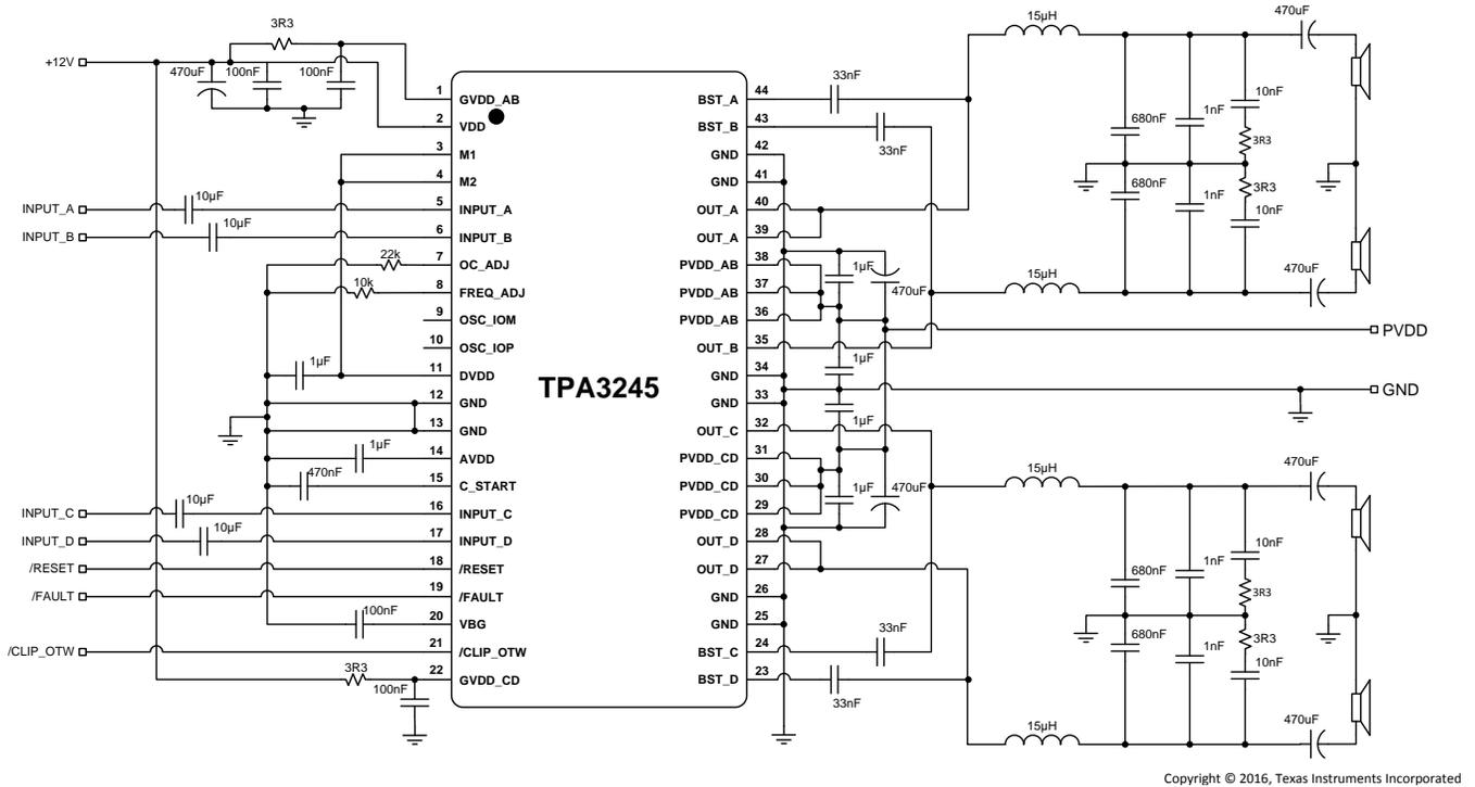
Figure 27. Typical Single Ended (1N) SE Application
