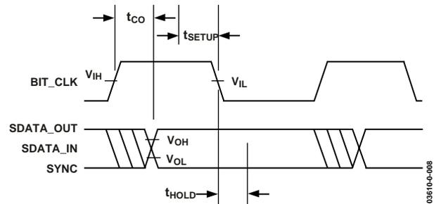
Figure 8. AC Link Low Power Mode Timing
