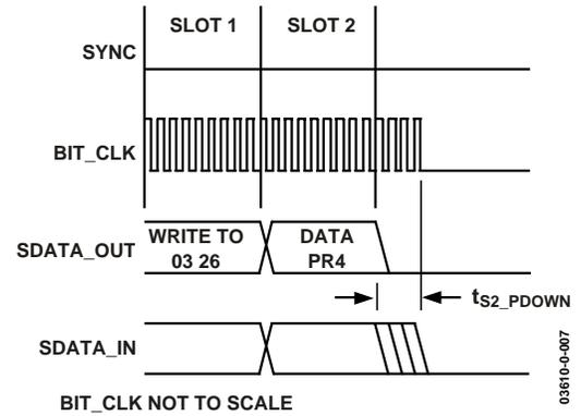
Figure 7. AC Link Low Power Mode Timing
