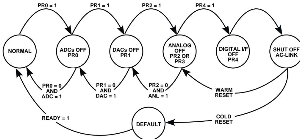
Figure 11. Example of AC '97 Power-Down/Power-Up Flow
