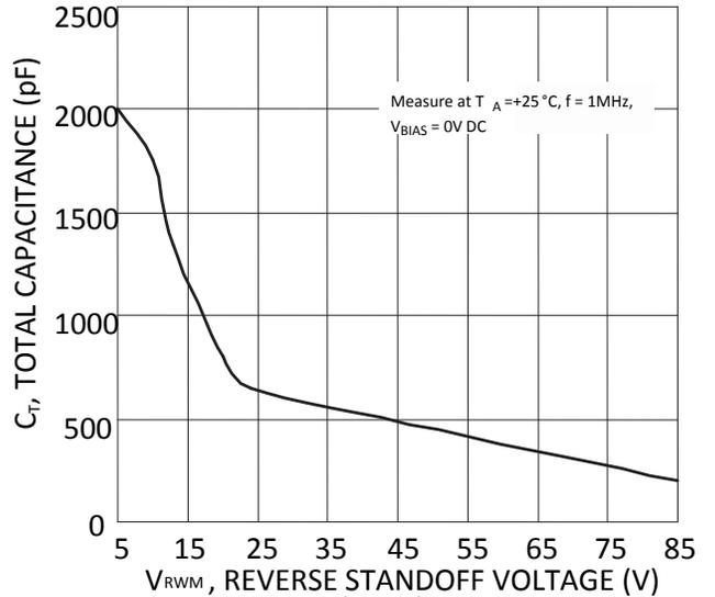
Fig. 2 Typical Total Capacitance vs. Reverse Standoff Voltage
