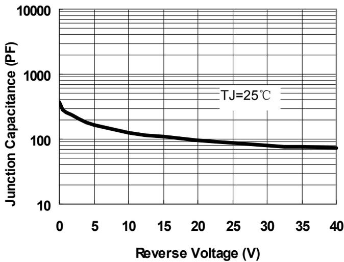
Fig.1-Typical Junction Capacitance
