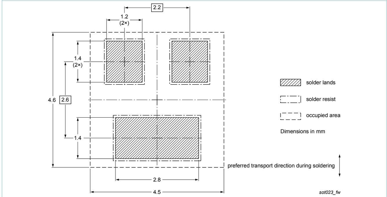
Fig. 20. Wave soldering footprint for TO-236AB (SOT23)
