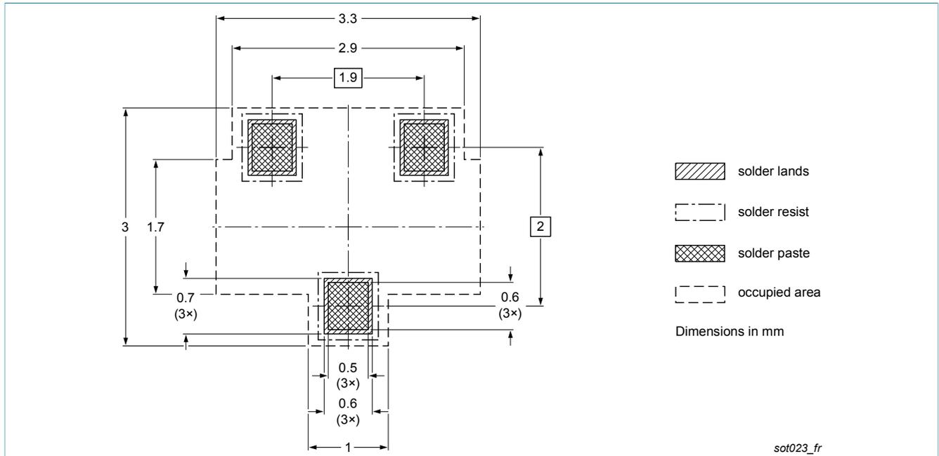
Fig. 19. Reflow soldering footprint for TO-236AB (SOT23)
