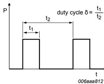
Fig. 17. Duty cycle definition
