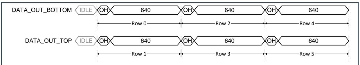
Only when 16 data outputs, running at 480 Mbps, are used, the frame rate of 30 fps can be achieved (default).
