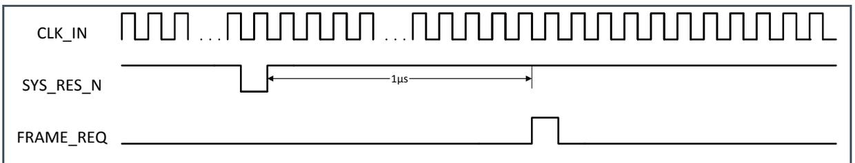
The on-board sequencer will be reset and all programming registers will return to their default start-up values when a falling edge is detected on the SYS\_RES\_N pin. After the reset there is a minimum time of 1 µs needed before a FRAME\_REQ pulse can be sent. All recommended register settings must be reloaded after a reset sequence.
