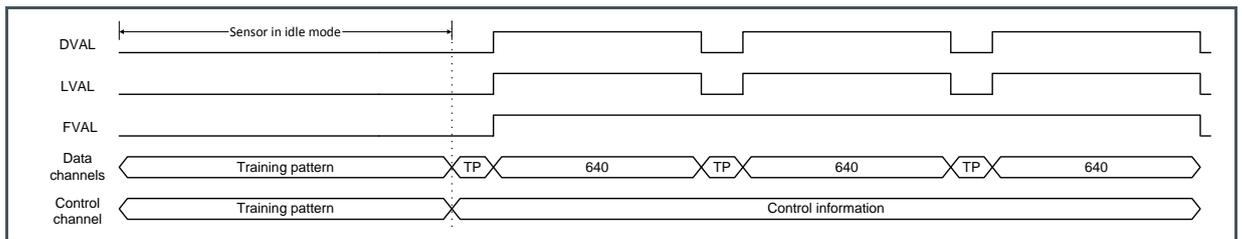
The LVDS outputs are not aligned with the LVDS output clock. Every channel (per odd/even side) has a skew of 600 ps compared to the previous channel. The control channel and both odd and even channels 1 are aligned with the clock. This skew will become larger than a LVDS clock period and therefore bit and word alignment is needed at the receiving side.
