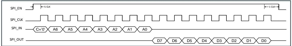
To indicate a read action over the SPI interface, the control bit on the SPI\_IN pin is made '0'. The address of the register being read out is sent immediately after this control bit (MSB first). After the LSB of the address bits, the data is launched on the SPI\_OUT pin on the falling edge of the SPI\_CLK. This means that the data should be sampled by the receiving system on the rising edge of the SPI\_CLK. The data comes over the SPI\_OUT with MSB first.
