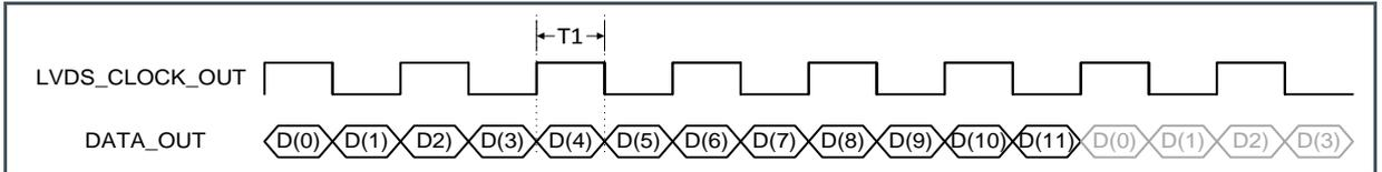
The time T1 in the diagram above is 1/12<sup>th</sup> of the period of the input clock (CLK\_IN) of the device. If a frequency of 40 MHz is used for CLK\_IN (max), this results in a 240 MHz LVDS\_CLOCK\_OUT.
