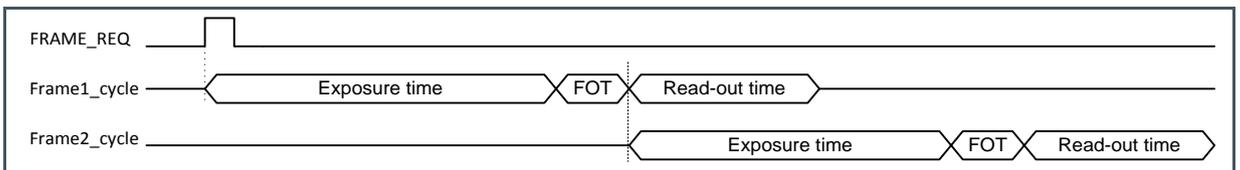
When the exposure time is shorter than the read-out time, the FOT and read-out of the next frame will start immediately after the read-out of the previous frame.
