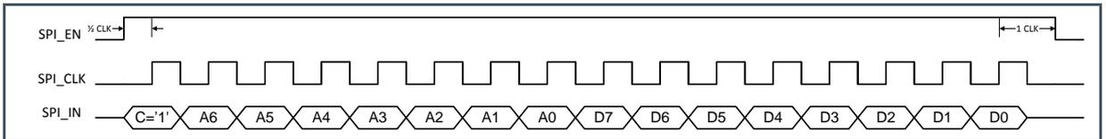
The data is sampled by the device on the rising edge of the SPI\_CLK. The SPI\_CLK has a maximum frequency of 20 MHz. The SPI\_EN signal has to be high for half a clock period before the first data bit is sampled. SPI\_EN has to remain high for 1 clock period after the last data bit is sampled.
