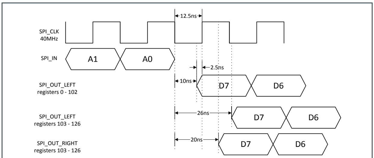
So when sampling on the rising SPI\_CLK edge it is advised to have a SPI\_CLK of 10 MHz maximum.
