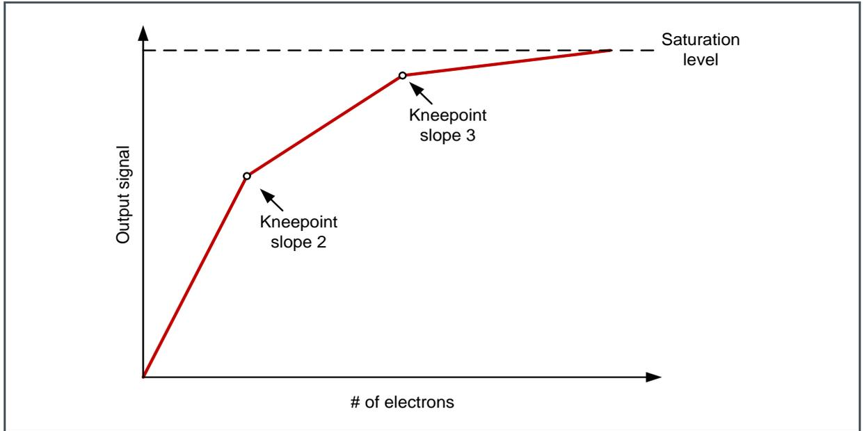
**Piecewise Linear Response with Internal Exposure Mode**
