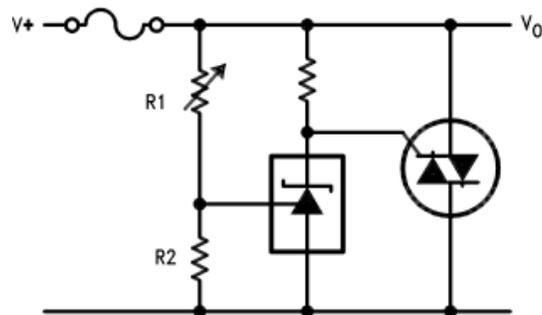
$$V_{LIMIT} \approx \left( 1 + \frac{R_1}{R_2} \right) V_{REF}$$
