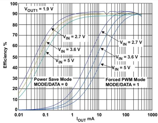
Figure 22. Efficiency TPS62404 VOUT1 = 1.9V, DEF\_1 = HIGH
