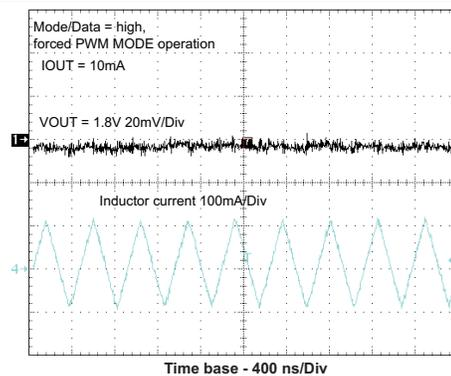
Figure 31. Output Voltage Ripple In Forced PWM Mode
