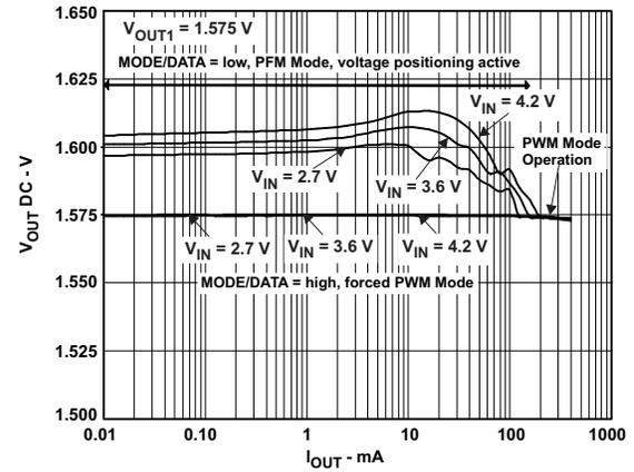
Figure 29. DC Output Accuracy  $V_{OUT1} = 1.575V$ ,
