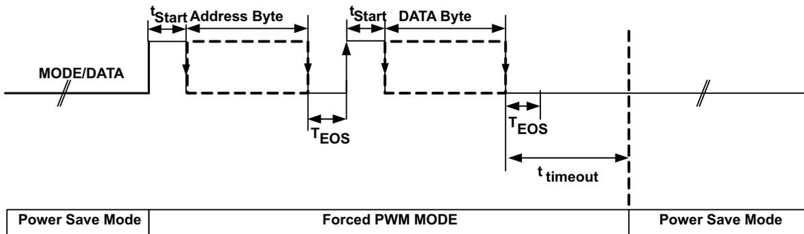
Figure 13. MODE/DATA Pin: Power Save Mode/Interface Communication
