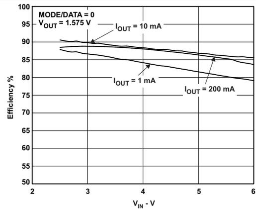
Figure 23. Efficiency vs V\_IN
