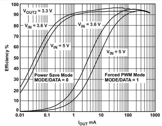
Figure 19. Efficiency TPS62400 VOUT 2 = 3.3V
