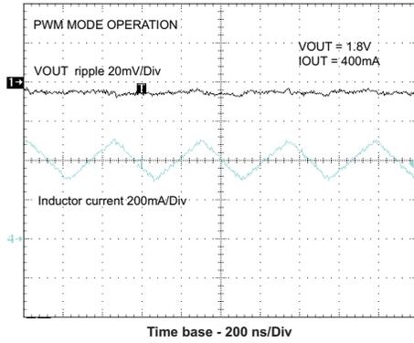
Figure 32. Output Voltage Ripple In PWM Mode
