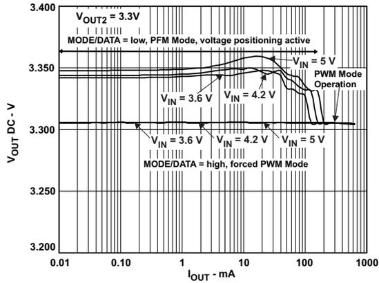
Figure 26. DC Output Accuracy  $V_{OUT2} = 3.3V$
