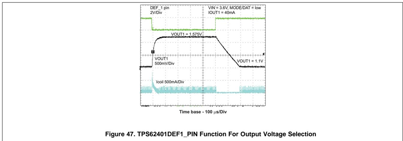
Figure 47. TPS62401DEF1\_PIN Function For Output Voltage Selection
