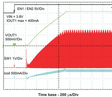
Figure 37. Startup Timing One Converter
