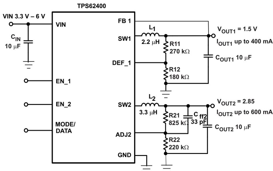
Figure 15. Typical Application Circuit 1.5V/2.85V Adjustable Outputs
