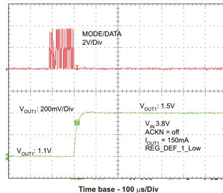
Figure 41.  $V_{OUT1}$  Change With Easyscale
