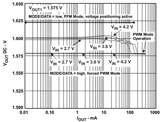
Figure 28. DC Output Accuracy  $V_{OUT1} = 1.575V$ ,
