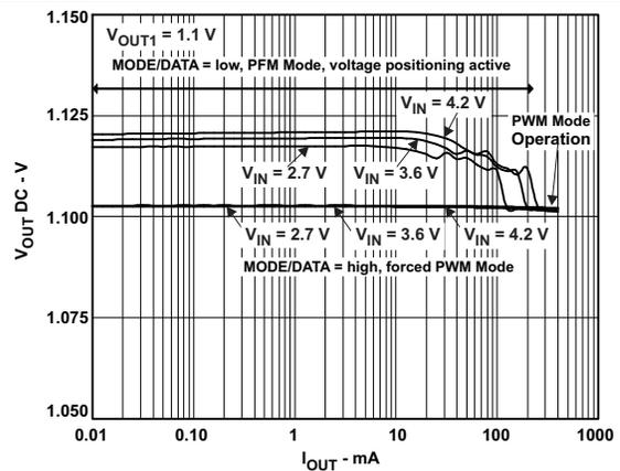
Figure 25. DC Output Accuracy VOUT1 = 1.1V
