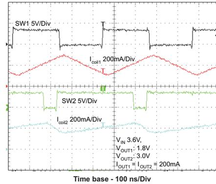
Figure 39. Typical Operation  $V_{IN} = 3.6V$ ,
