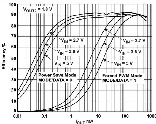
Figure 18. Efficiency VOUT 2 = 1.8V
