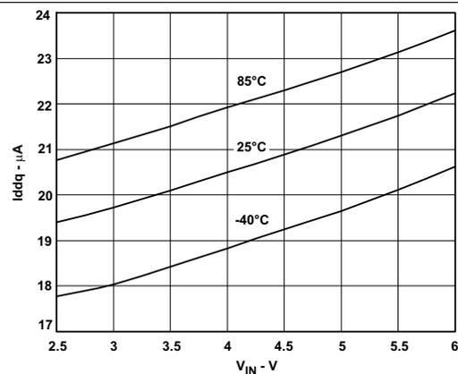
Figure 2.  $I_q$  For One Converter, Not Switching
