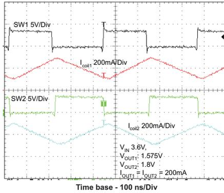
Figure 38. Typical Operation  $V_{IN} = 3.6V$ ,
