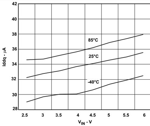
Figure 3. I<sub>q</sub> For Both Converters, Not Switching
