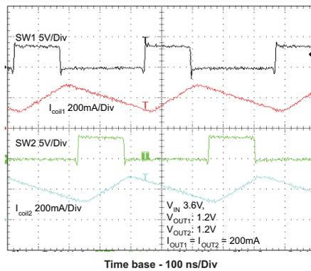
Figure 40. Typical Operation  $V_{IN} = 3.6V$ ,
