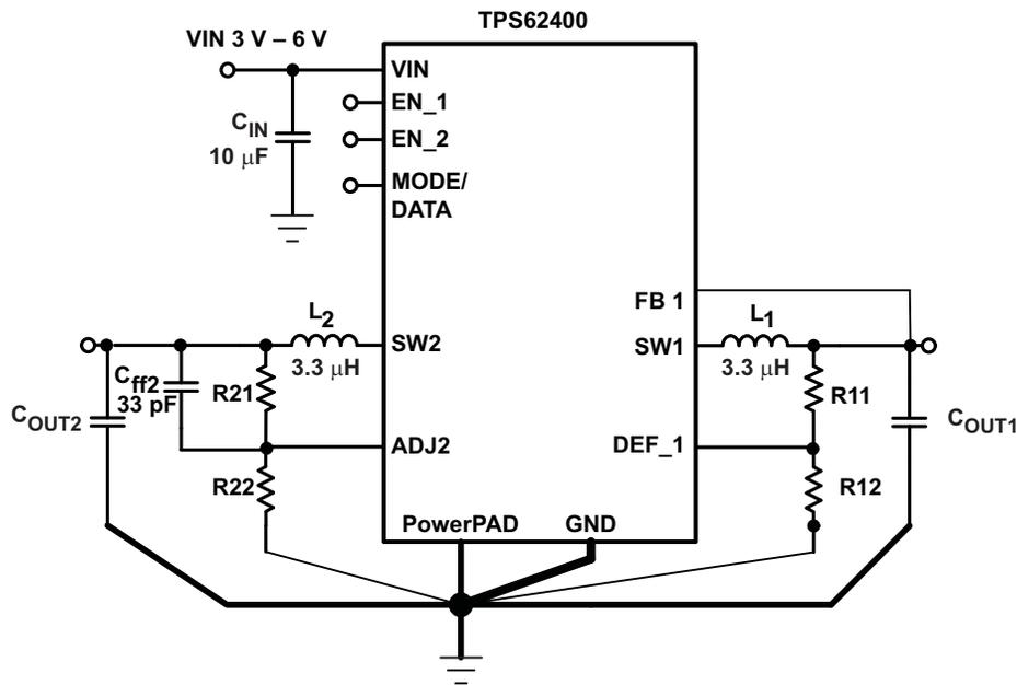
Figure 48. Layout Diagram
