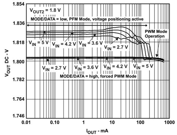
Figure 27. DC Output Accuracy  $V_{OUT2} = 1.8V$
