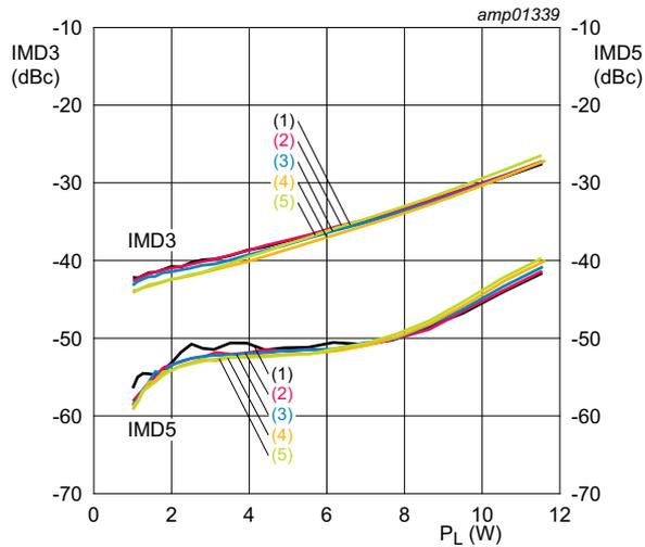
2-Tone signal with 100 kHz carrier separation:  $V_{DS} = 13.6\text{ V}$ ;  $I_{Dq} = 500\text{ mA}$ .
