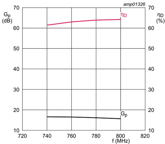
$V_{DS} = 13.6 \text{ V}$ ;  $I_{Dq} = 100 \text{ mA}$ ;  $P_L = 25 \text{ W}$ .
