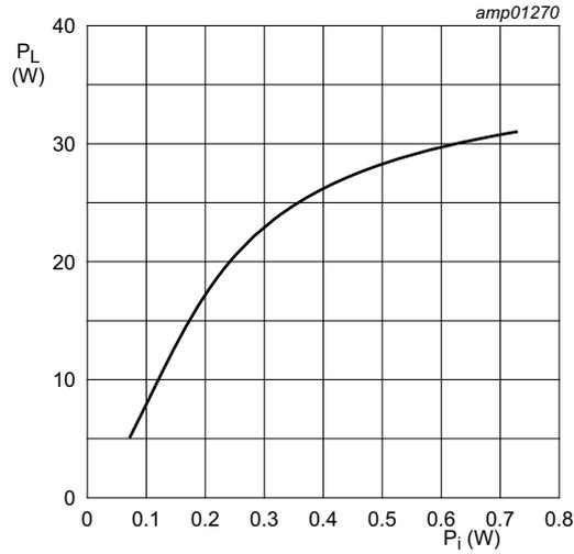
$V_{DS} = 13.6 \text{ V}$ ;  $f = 520 \text{ MHz}$ ;  $I_{Dq} = 45 \text{ mA}$ .
