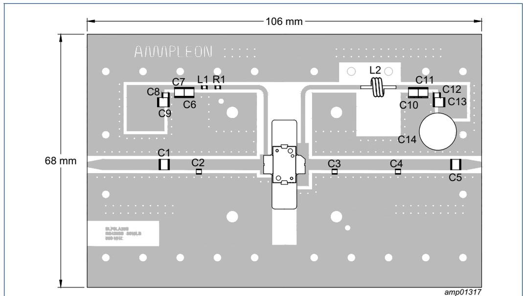
Printed-Circuit Board (PCB): Rogers RO4350B; height = 0.762 mm.
