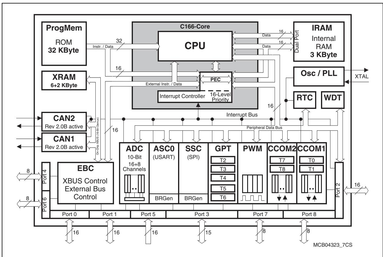
**Figure 3 Block Diagram**
