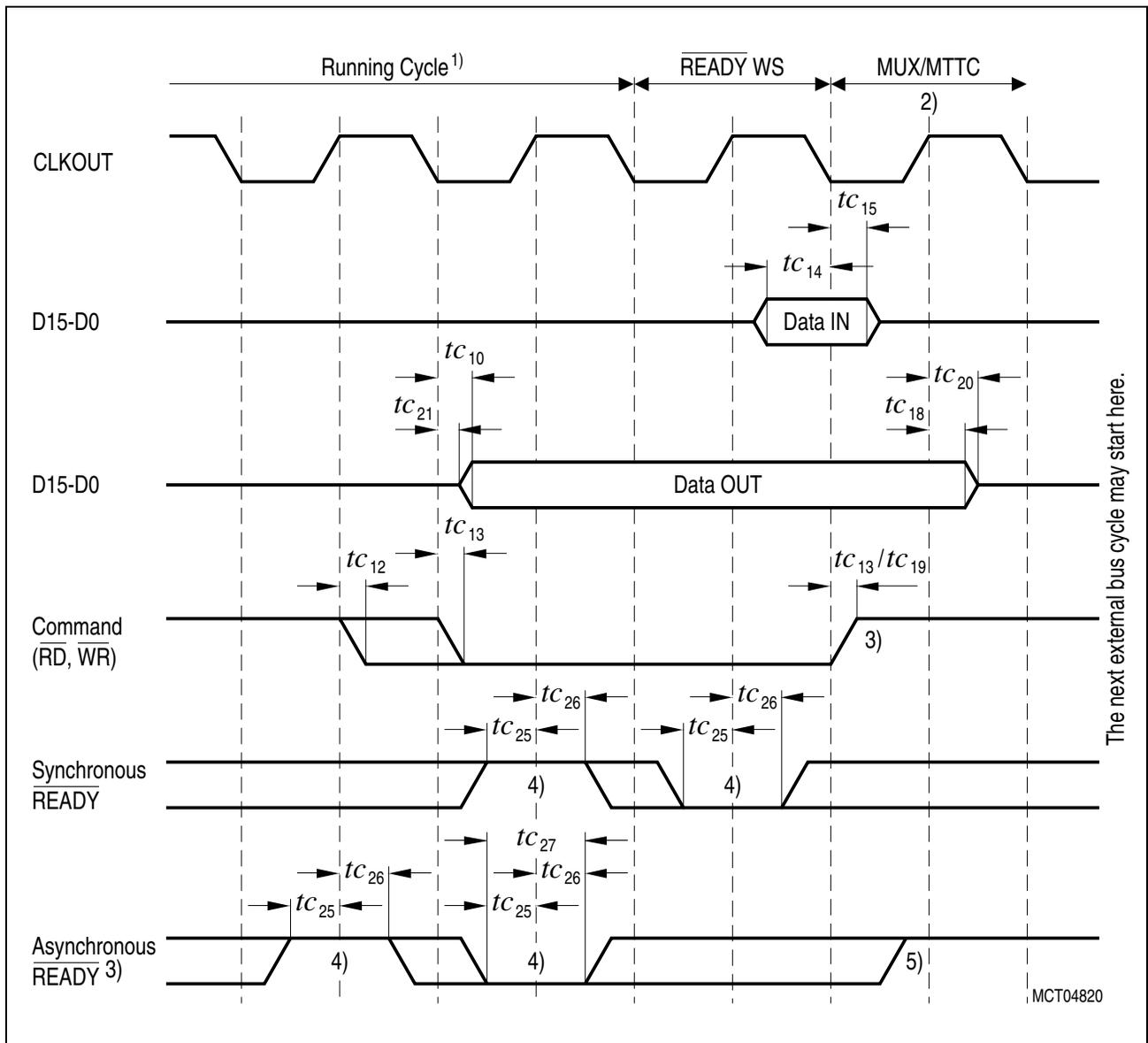
Figure 21  $\overline{\text{READY}}$  Timing
