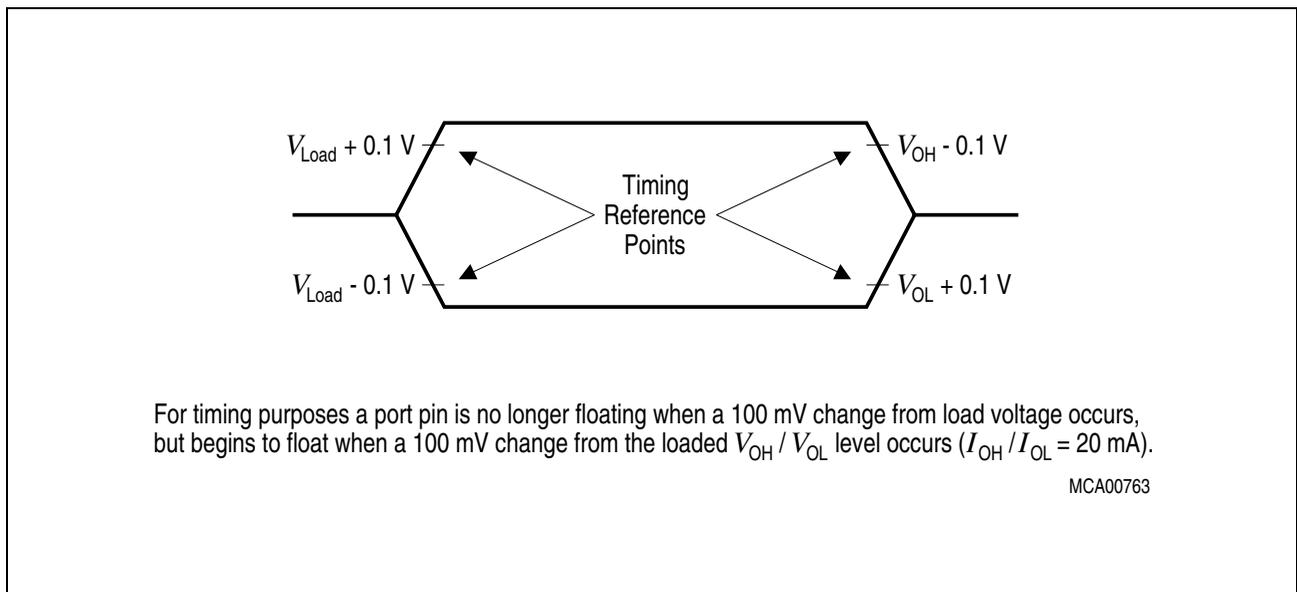
**Figure 15** Float Waveforms
