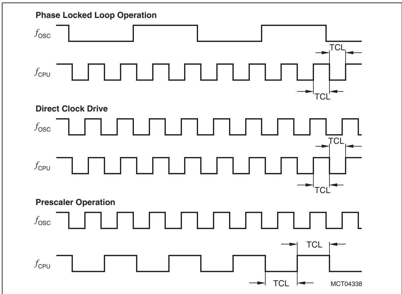
**Figure 11** Generation Mechanisms for the CPU Clock
