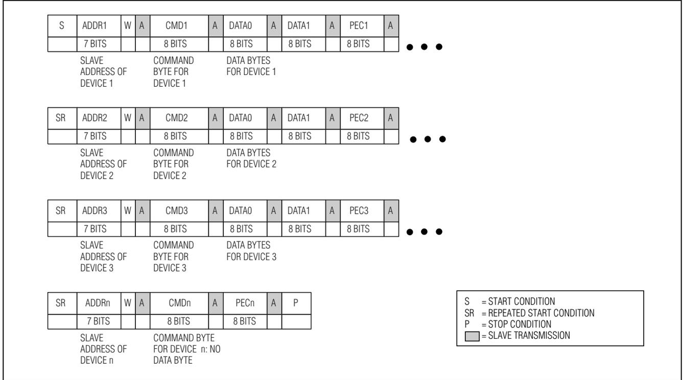
Figure 15. SMBus Group Command Protocol with PEC
