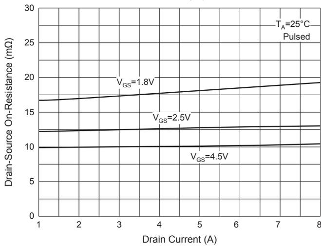
Fig. 4 -  $R_{DS(ON)} - V_{GS}$
