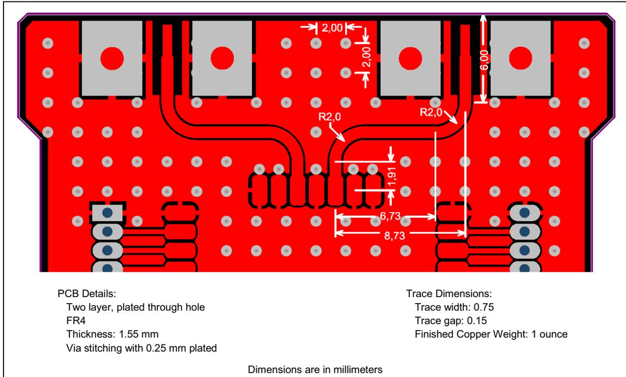
**FIGURE 5-2: RF TRACE ROUTING (BOTTOM LAYER)**
