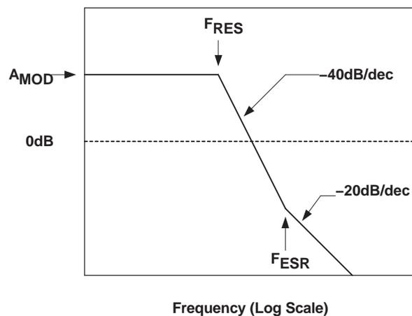
**Figure 20. Power Stage Frequency Response Straight Line Approximation**
