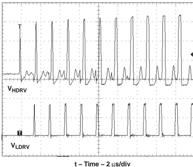
Figure 16. MOSFET Drivers at Beginning of Soft Start
