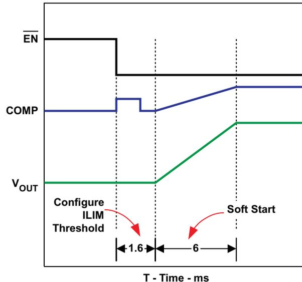
Figure 15. Startup with  $V_{\text{REFIN}} = 1.5 \text{ V}$
