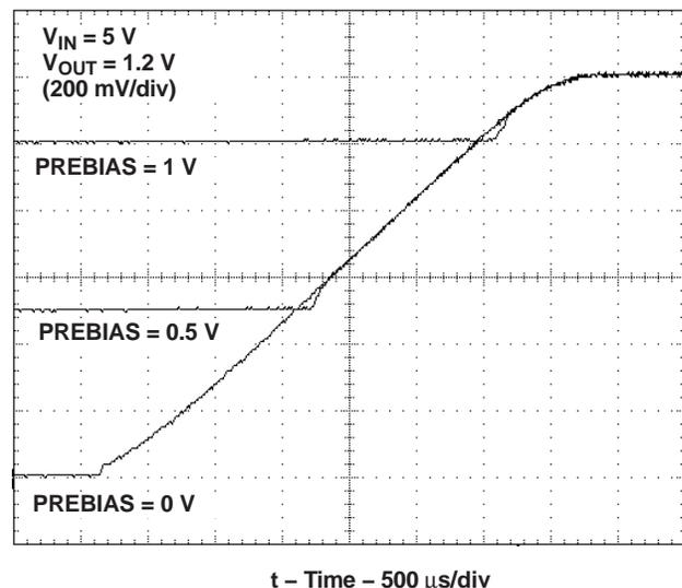
Figure 17. Startup Waveforms; VREFIN = 0.6 V
