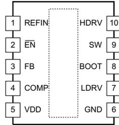
Figure 13. DRC Package Terminal Configuration (Top View)
