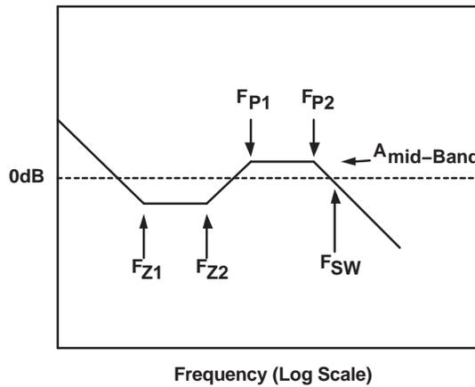
Figure 21. Error Amplifier Frequency Response Straight Line Approximation
