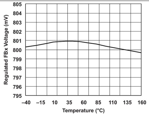
Figure 16. Regulated FBx Voltage vs Temperature (Buck)
