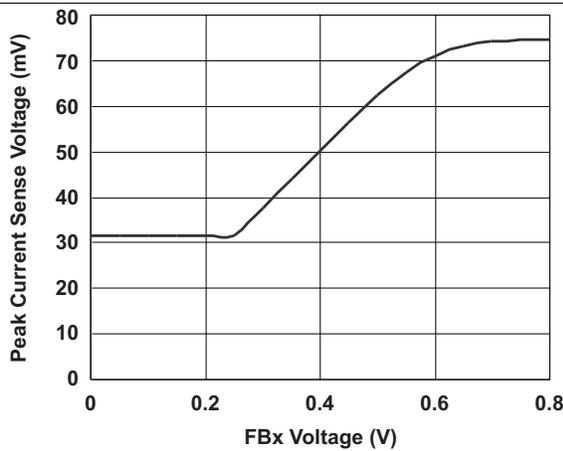
Figure 15. Foldback Current Limit (Buck)
