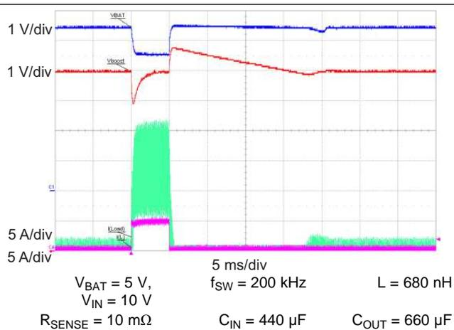
Figure 8. Load Step Response (Boost)
