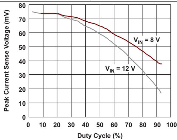
Figure 17. Current Limit vs Duty Cycle (Buck)
