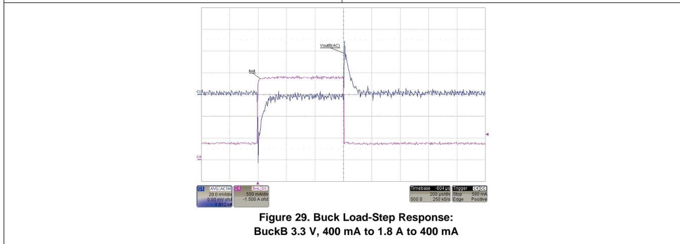
Figure 29. Buck Load-Step Response: BuckB 3.3 V, 400 mA to 1.8 A to 400 mA
