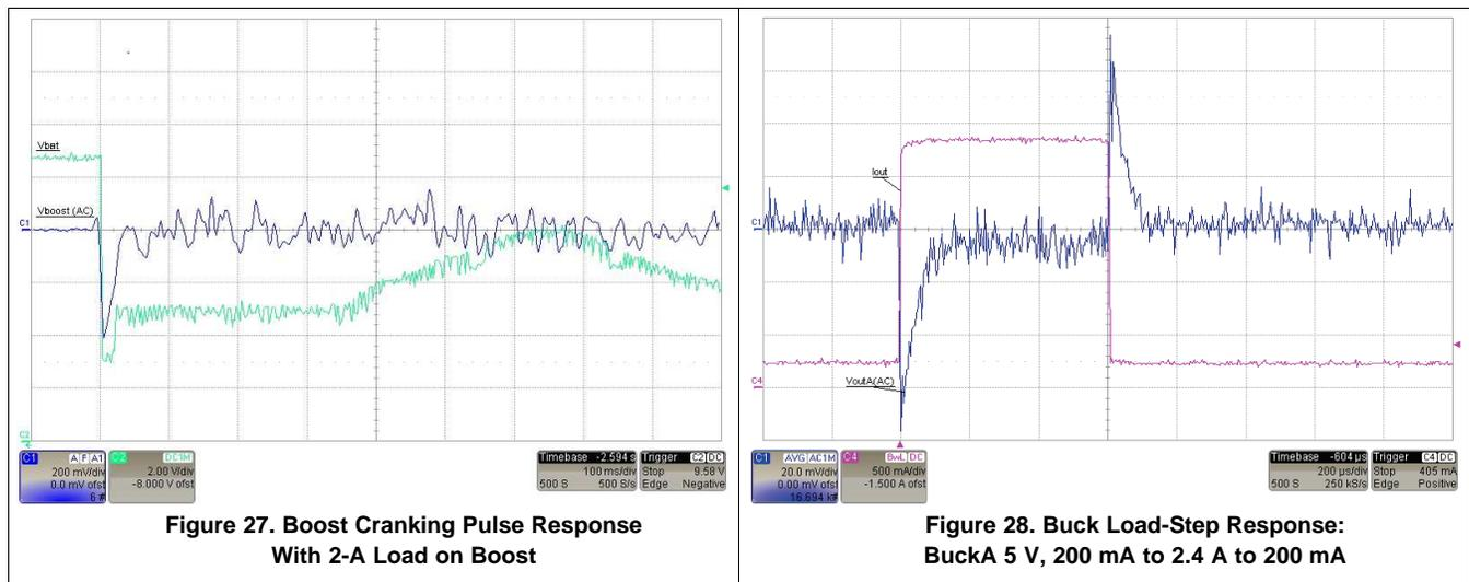
Figure 27. Boost Cranking Pulse Response With 2-A Load on Boost
