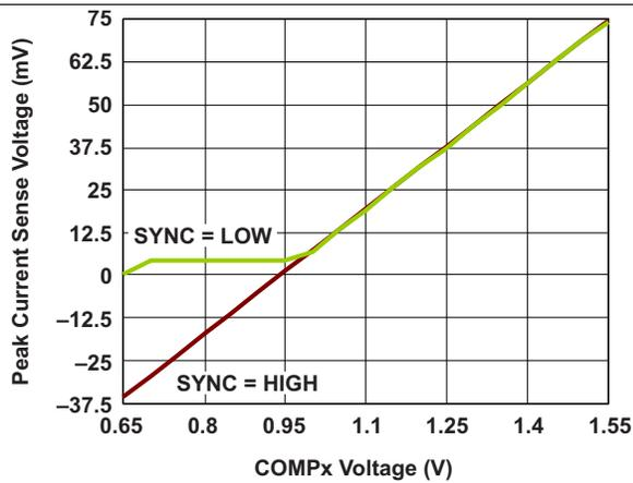
Figure 13. BUCKx Peak Current Limit vs COMPx Voltage
