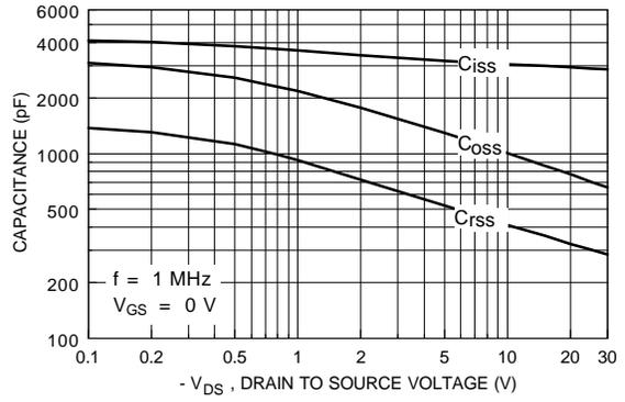
**Figure 8. Capacitance Characteristics.**
