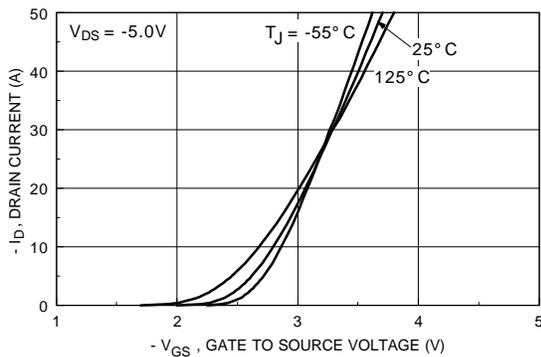
Figure 5. Transfer Characteristics.
