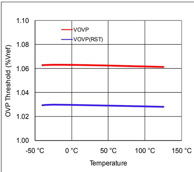
**Figure 11: Over Voltage Protection Thresholds vs. Temperature**
