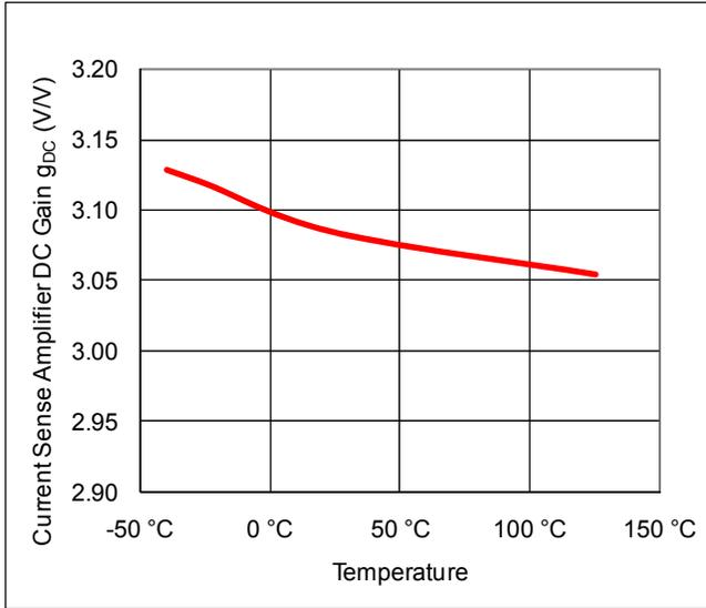
**Figure 9: Current Amplifier DC Gain vs. Temperature**
