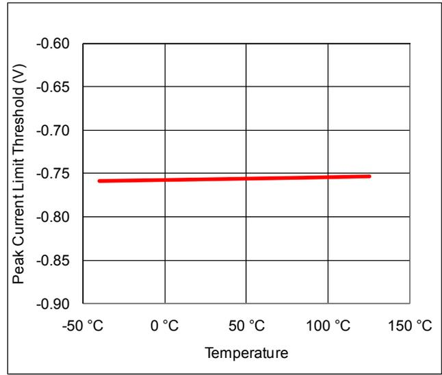
**Figure 10: Peak Current Limit Threshold  $V_{ISNS(PK)}$  vs. Temperature**
