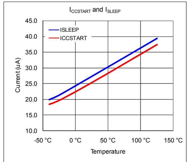
**Figure 4: Startup Current and Sleep Current vs. Temperature**
