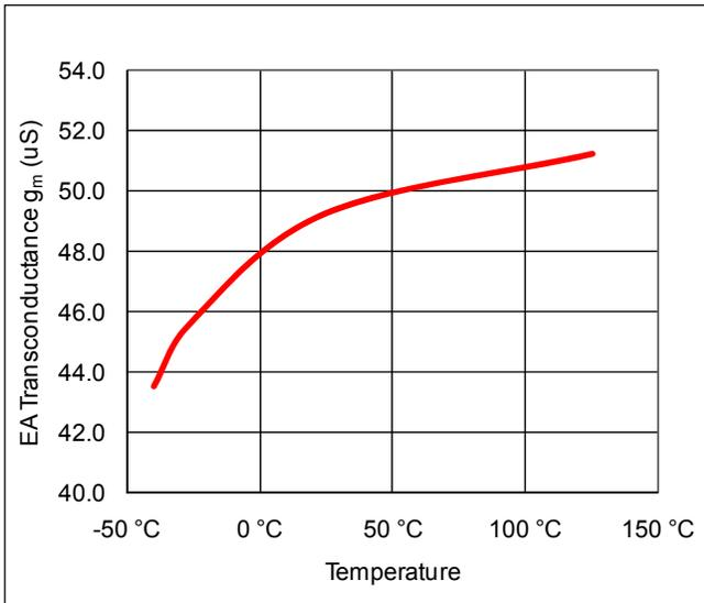
**Figure 7: Voltage Error Amplifier Transconductance vs. Temperature**
