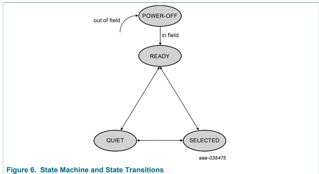
**Figure 6. State Machine and State Transitions**
