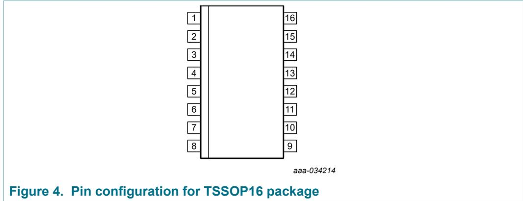
Figure 4. Pin configuration for TSSOP16 package
