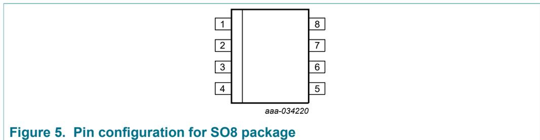
Figure 5. Pin configuration for SO8 package
