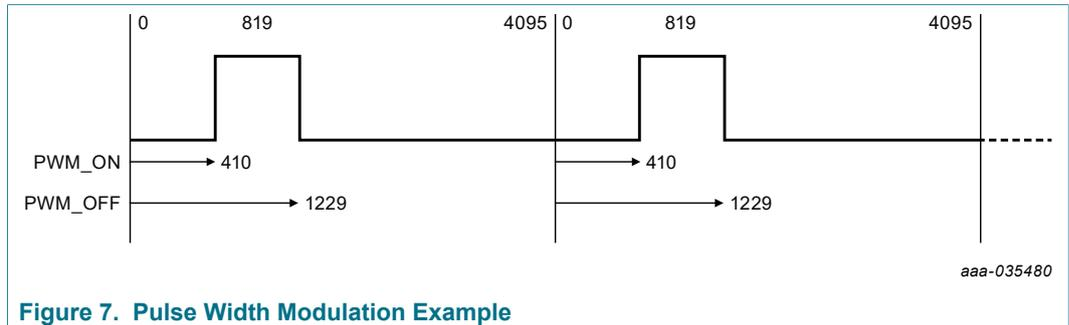
Figure 7. Pulse Width Modulation Example
