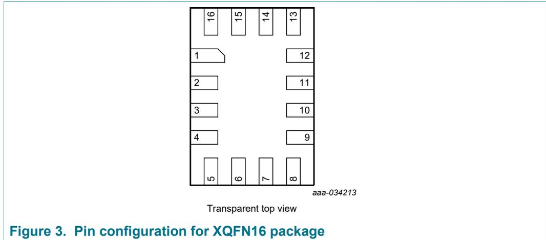
**Figure 3. Pin configuration for XQFN16 package**
