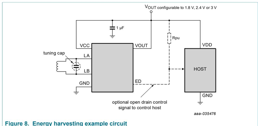
Figure 8. Energy harvesting example circuit
