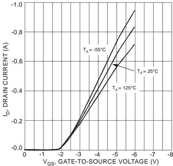
Fig. 3 Drain Current vs. Gate Source Voltage
