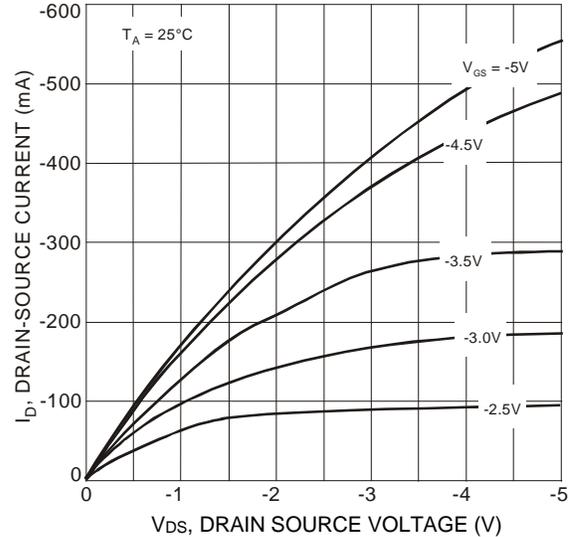
Fig. 2 Drain Source Current vs. Drain Source Voltage
