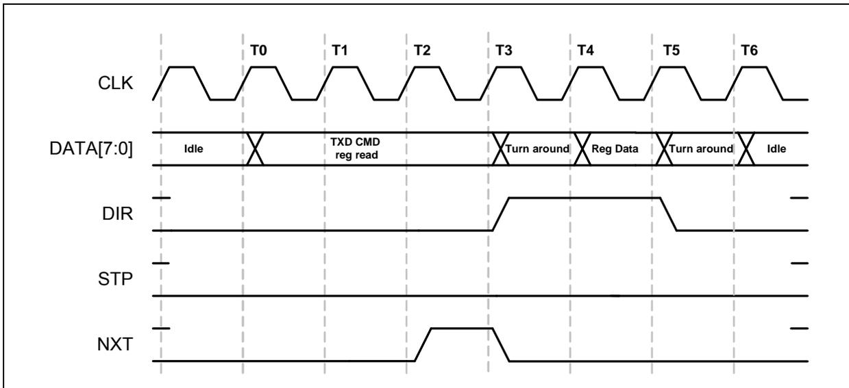
At T0, the Link will place the TX CMD on the data bus. At T2, the PHY will bring **NXT** high, signaling the Link it is ready to accept the data transfer. At T3, the PHY reads the TX CMD, determines it is a register read, and asserts **DIR** to gain control of the bus. The PHY will also de-assert **NXT**. At T4, the bus ownership has transferred back to the PHY and the
