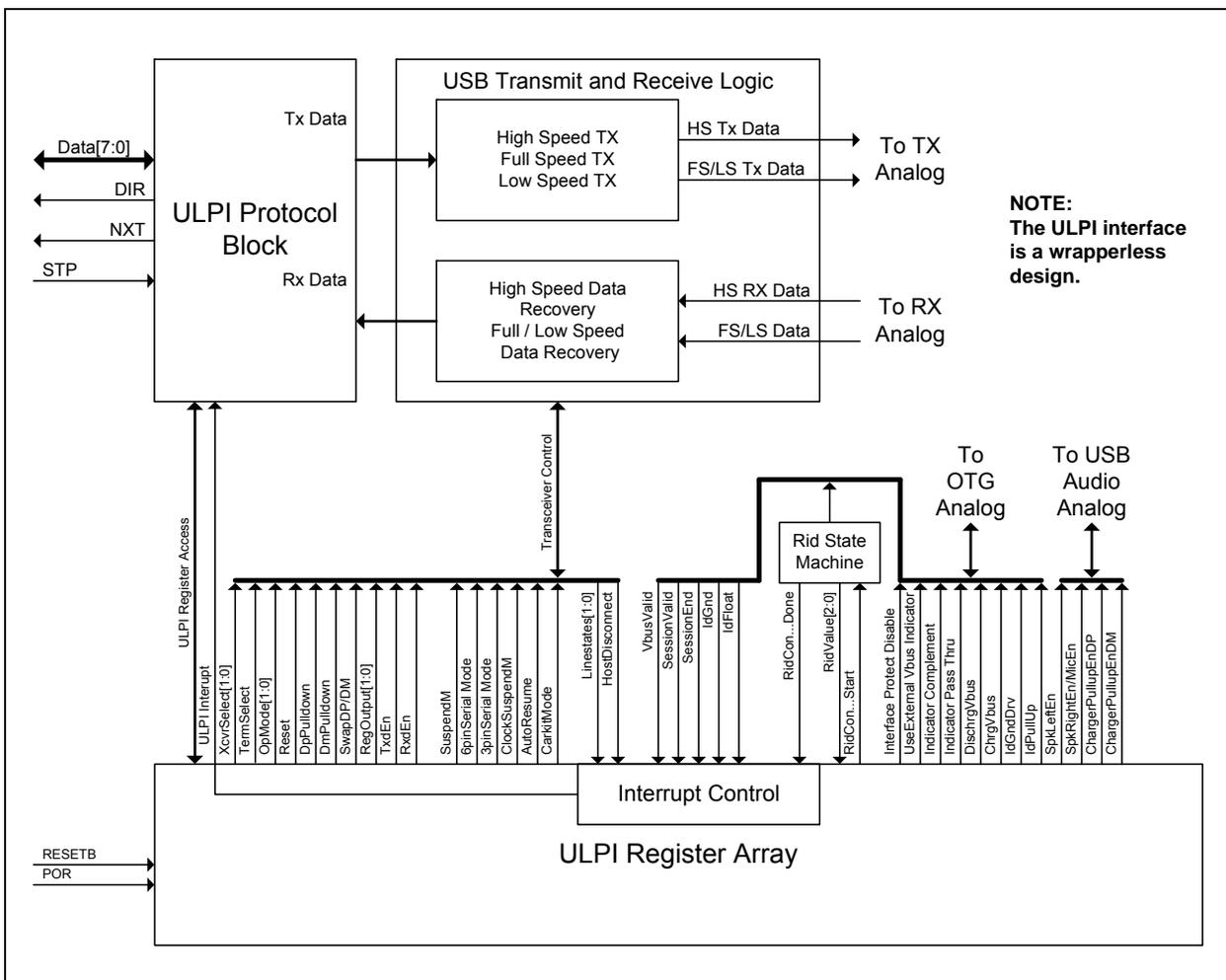
The advantage of a “wrapper-less” architecture is that the USB3333x has a lower USB latency than a design which must first register signals into the PHY’s wrapper before the transfer to the transceiver core. A low latency PHY allows a wrapper around a UTMI Link to be used and still make the required USB turn-around timing required by the USB 2.0 specification.
