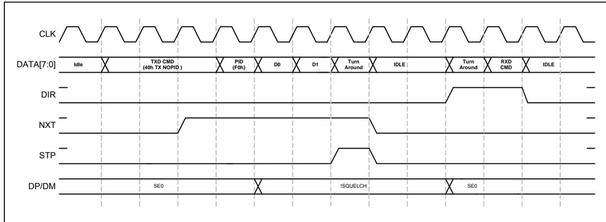
To send the 'F0' PID, the link will be required to use the TX CMD with NOPID to initiate the transmit and then follow up the TX CMD with the 'F0' PID. The data bytes follow as in a normal transmit, in *OpMode* 00b. The key difference is in that the link will have to send the PID the same as it would send a data packet. The USB333x is able to recognize the LPM transmit and correctly send the PID information.
