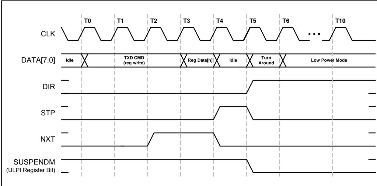
While in Low Power Mode, the Data interface is redefined so that the Link can monitor Linestate and the VBUS voltage. In Low Power Mode **DATA[3:0]** are redefined as shown in [Table 6-7](#). Linestate[1:0] is the combinational output of the Single-Ended Receivers. The “int” or interrupt signal indicates an unmasked interrupt has occurred. When an unmasked interrupt or linestate change has occurred, the Link is notified and can determine if it should wake-up the PHY.
