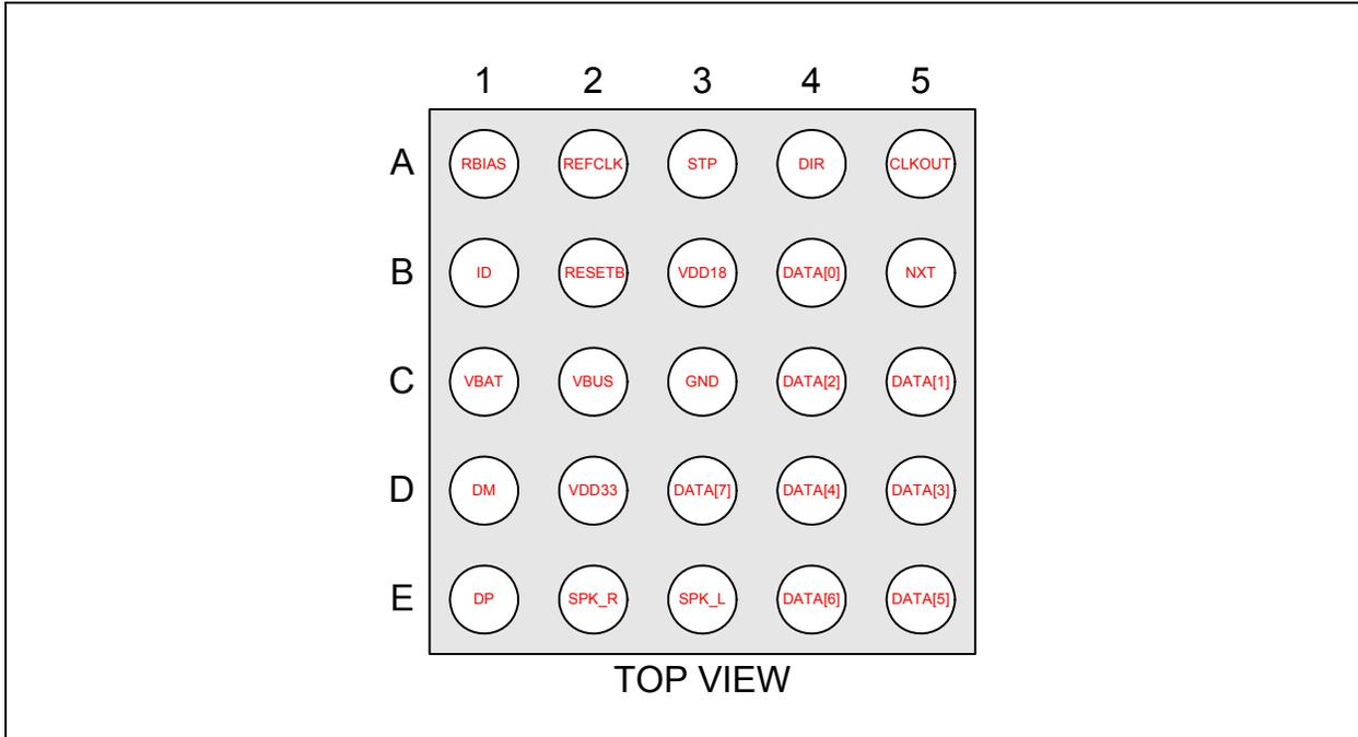
FIGURE 2-2: USB3330 BALL LOCATIONS - TOP VIEW
