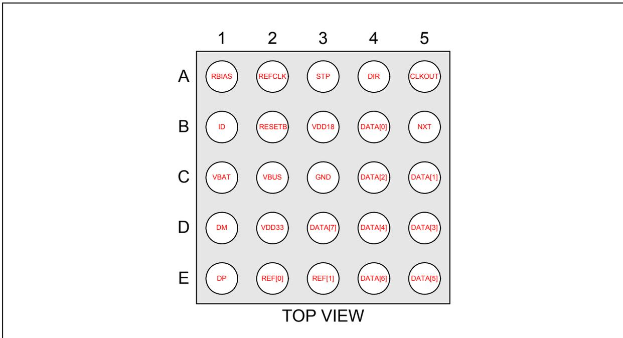
**FIGURE 2-3: USB3333 BALL LOCATIONS - TOP VIEW**
