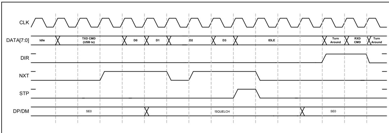
During transmit the PHY will use **NXT** to control the rate of data flow into the PHY. If the USB333x pipeline is full or bit-stuffing causes the data pipeline to overflow **NXT** is de-asserted and the Link will hold the value on Data until **NXT** is asserted. The USB Transmit ends when the Link asserts **STP** while **NXT** is asserted.
