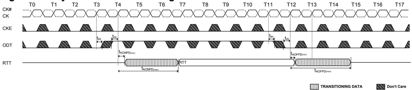
**Figure 73. Synchronous to asynchronous transition during Precharge Power Down (with DLL frozen) entry (AL = 0; CWL = 5; tANPD = WL - 1 = 4)**
