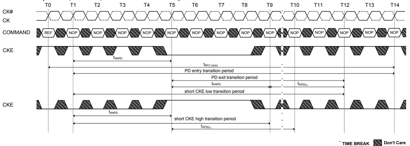
**Figure 77. Power-Down Entry, Exit Clarifications-Case 1**
