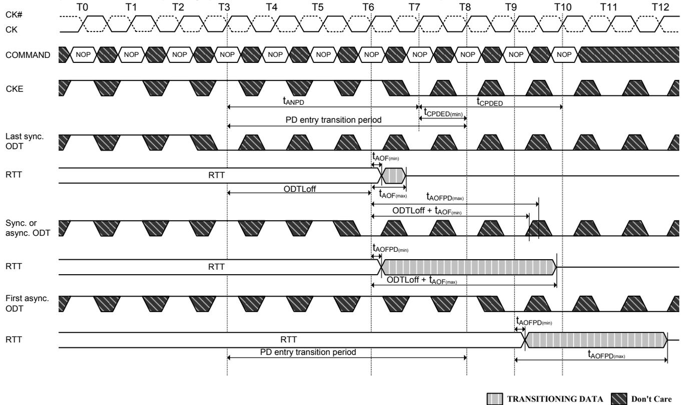
**Figure 74. Synchronous to asynchronous transition after Refresh command**
