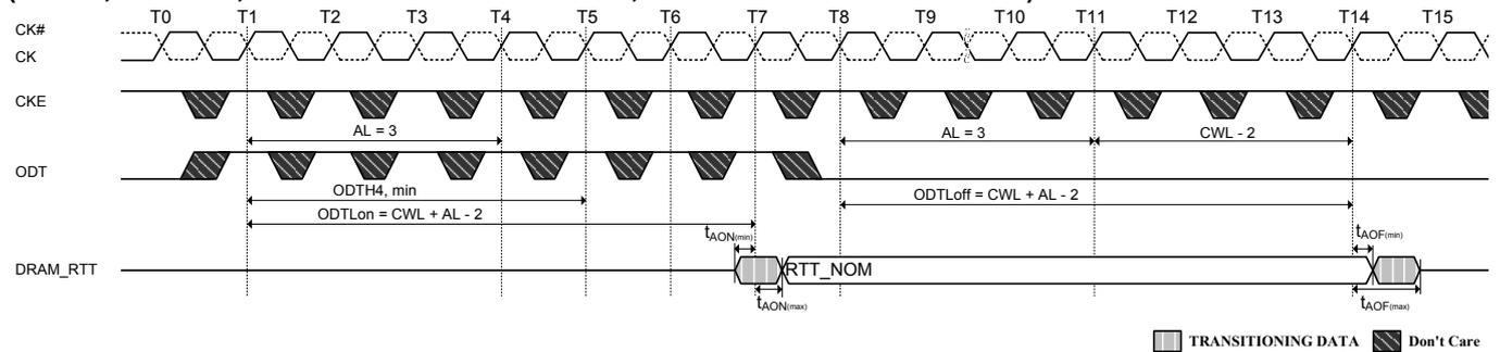
**Figure 66. Synchronous ODT example with BL = 4, WL = 7**
