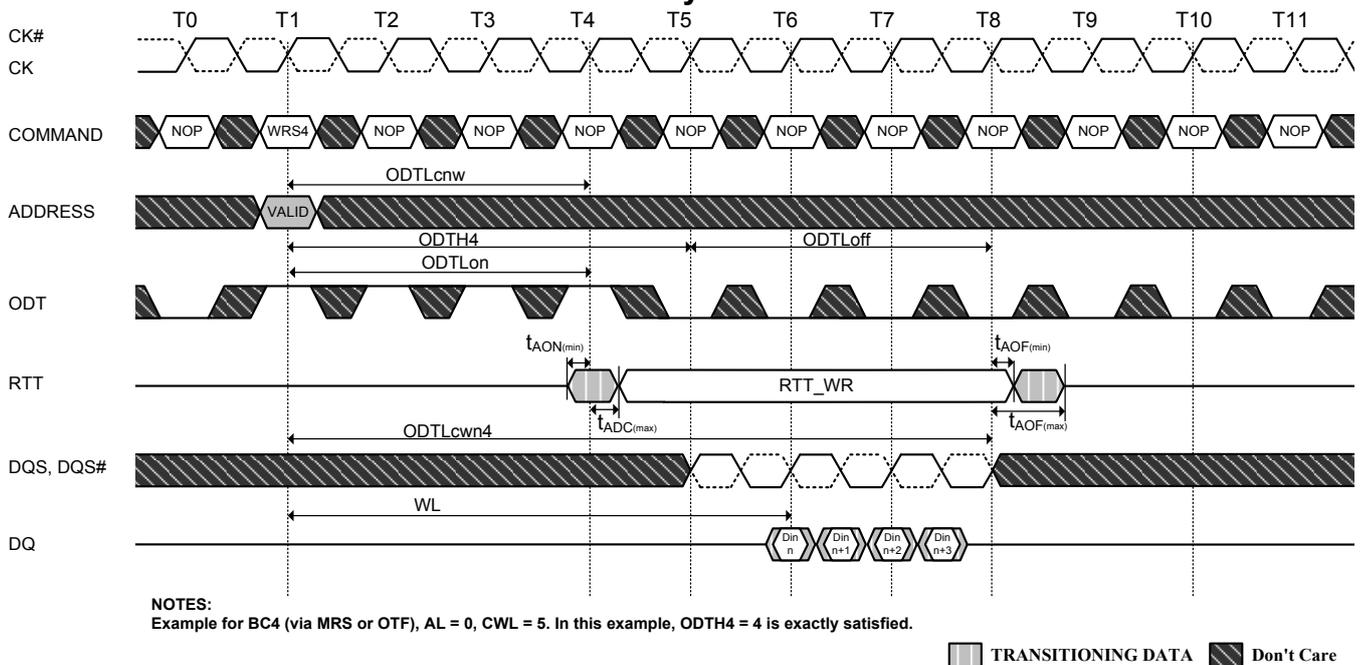
**Figure 72. Asynchronous ODT Timings on DDR3 SDRAM with fast ODT transition**
