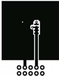
a) 50  $^\circ\text{C}/\text{W}$  when mounted on a 1 in<sup>2</sup> pad of 2 oz copper.
